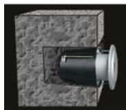
• Installation with clips embedded into sleeve, fix on the concrete wall
